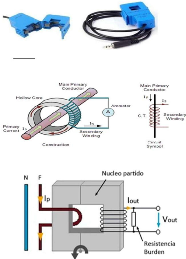
A current transformer seeks to generate an intensity in the secondary that is proportional to the intensity that passes through the primary. For this, it is desired that the primary is formed to reduced number of turns. The SCT-013 sensors are small current transformer. Current transformers are instruments widely used for measuring elements.
