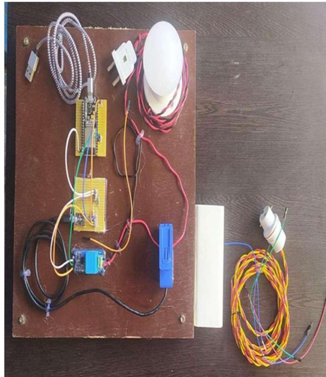
The output generated by giving power supply to the load, the current voltage value can be verify using the standard multimeter. The output data can be monitored in blynk application and the voltage current and the power value displayed in numerical format.
